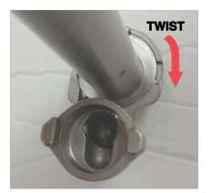
2) Once Part B Tabs are in the Notches of Part E press them together tightly and twist Part B Clockwise until both tab's fit under the lips of Part E.
